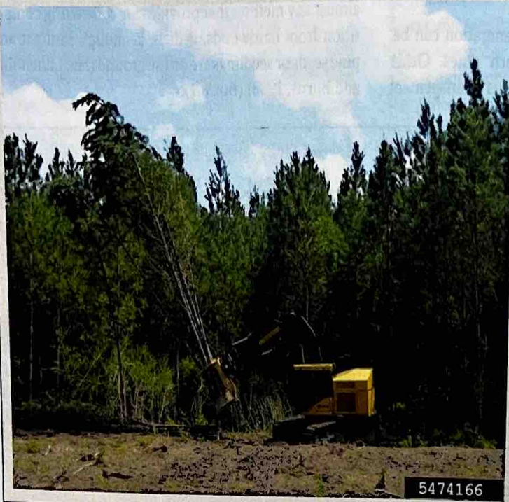
Box 8.1 Figure 2 Fifteen-year-old loblolly pine ( Pinus taeda ) being harvested in a strip clearcut. Slash is being chipped and the soil surface is being scarified for seed dispersal from the adjacent stand. Source: US Forest Service.
